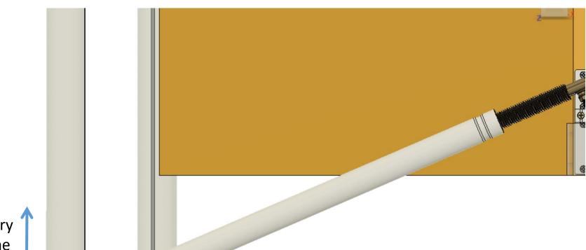
Vertical placement of jack clamp will vary depending on the maximum angle of the front tube.
