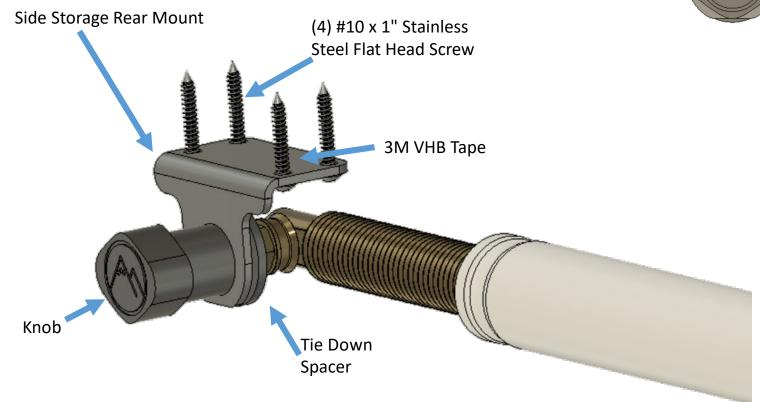
\*\*Please note: The 3M VHB tape used on the front and rear side storage hanger mounts is very strong and repositioning the mounts after they have been fixed to the camper is not advised. When installing the mounts, be sure of placement before removing the adhesive backing and attaching the mounts with the screws.
